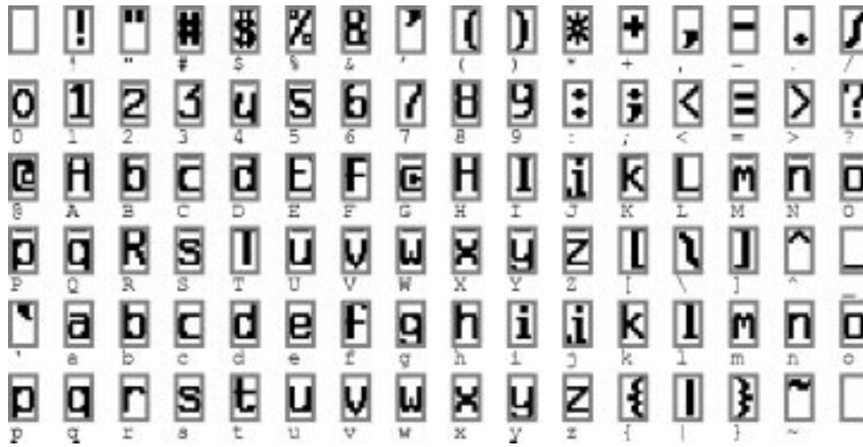
Fig. 3. Initial parameters of the output RBF's for recognizing the full ASCII set.
